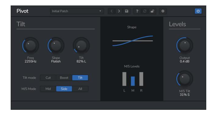
Pivot is a mid/side tilt equaliser, meaning that you can adjust the amplitude of the frequency spectrum like a seesaw, with the option to apply the tilt to the mid and side channels. Move the tilt knob to the left, and the low end becomes quieter as the high end becomes louder; turn it to the right for the opposite effect.
